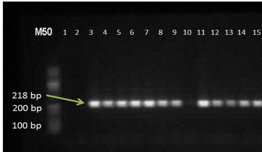
Fig. 2: Electrophoresis showing the results of Conventional PCR reaction. Line 1 and 15 are negative and positive control, respectively; Line 2 and 10 are negative (positive in microscopic methods); Line 3-9, 11-14 correspond to N. ceranae ; M-Molecular marker 50 bp
