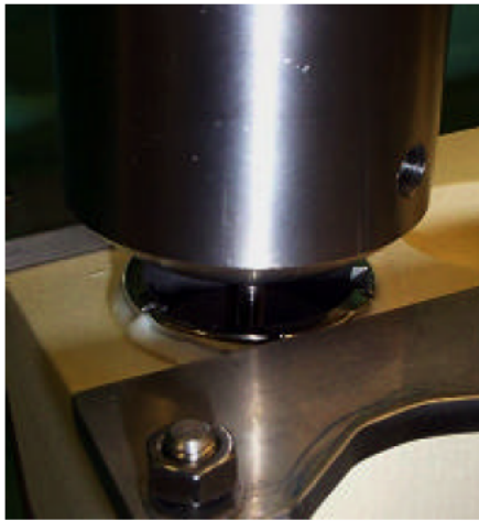
Fig.7: Testdevice for pullout-test
