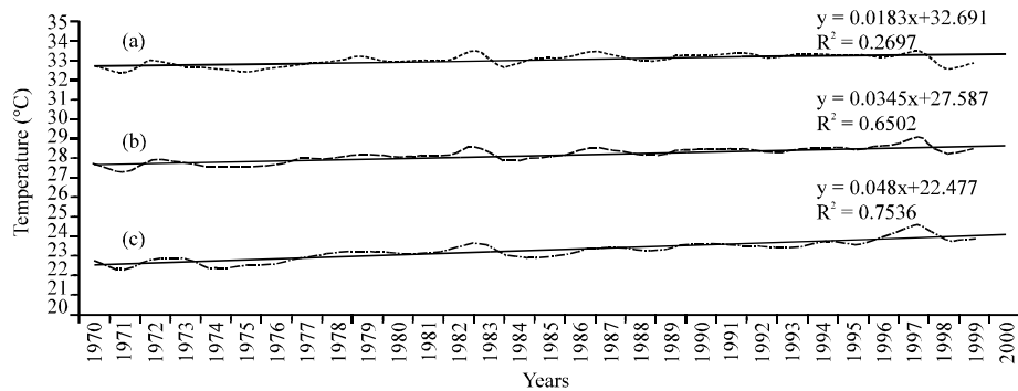
Fig. 1: Annual surface maximum, minimum and mean annual average temperature trends of Ipoh during 1970-2000; a) Maximum temperature; b) Annual average temperature; c) Minimum temperature (Anomly of mean, maximum, minimum and average temperature (1970-2000)); Anomly (°C)
