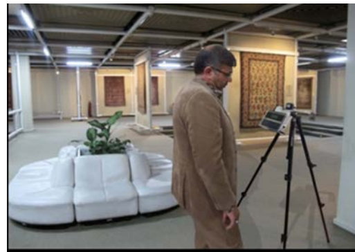
Fig. 1: LSI for measuring atmospheric pollutants
