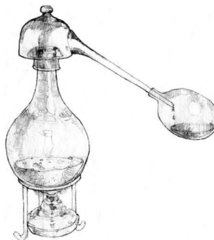
Fig. 1: Alembic; Distillation apparatus from 8th century Arabic treaties on Chemistry. The 1001 inventions Muslim heritage in our world, 2007 by Salim T. S. Al-Hassani. London, UK. Foundation for Science Technology and Civilization (FSTC)
