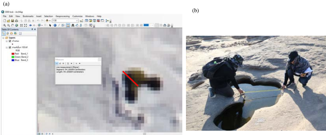
Fig. 3: (a) Measuring the width of the pothole from an unmanned aerial vehicle by ArcGIS program and (b) Measuring the width of the pothole by field study
