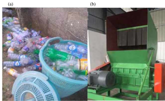
Fig. 4(a-b): (a) Washed PET bottles and (b) PET Plastic crushing machine
