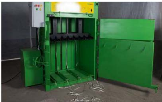
Fig. 12: Waste plastic/aluminum cans bailing machine
