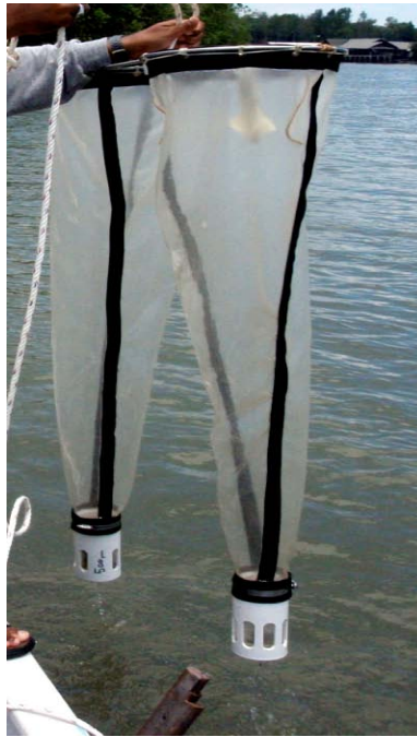
Fig. 2: Bongo net (Mesh size: 500 \mu\text{m} , mouth diameter: 0.3 m and length: 1.3 m) was used to catch fish larvae in the seagrass-mangrove ecosystem of Gelang Patah, Johor
