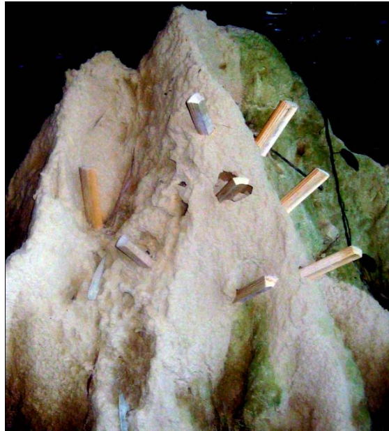
Fig. 8: Termite mound test of bamboo samples
