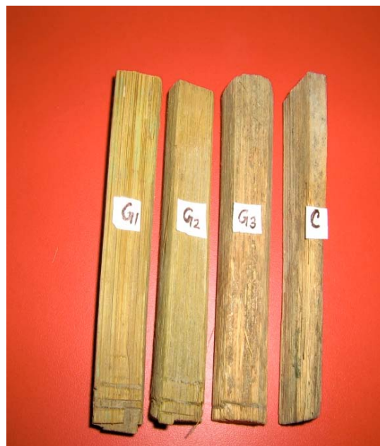
Fig. 8: Termite mound test of bamboo samples
