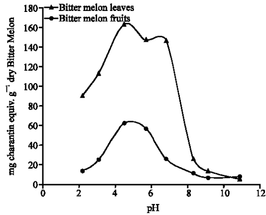
Fig. 1: Effect of pH on charantin extraction at 50 and 70% ethanol, 70.24 and 80.34°C and a time of contact of 60 and 70 h for fruit and leaves, respectively
