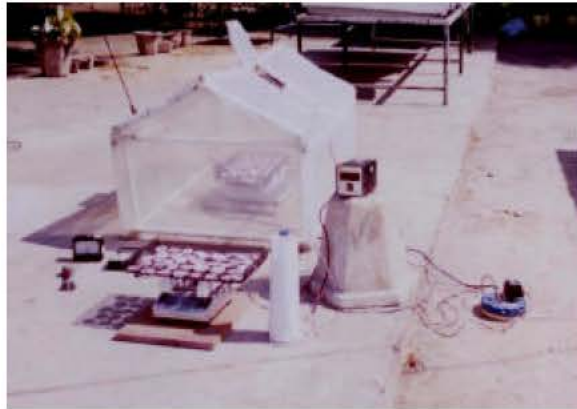
Fig. 1: Onion drying under opens sun and natural convection mode in greenhouse
