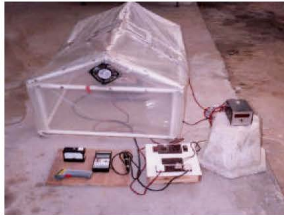
Fig. 2: Onion drying under force convection mode in greenhouse
