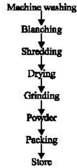
Fig. 7: Flow chart for preparation of aonla shreds
