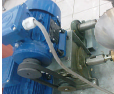
Fig. 12: Motor and gearbox for jam's screw
