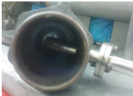
Fig. 8: Cross section view of dough's nozzle horn
