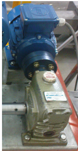
Fig. 13: Motor and gearbox for dough's screw
