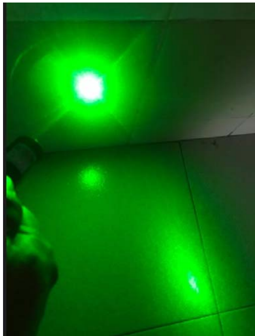
Fig. 6: Reflection of many light spots/rings on the floor can be observed from a bundle of laser beams
