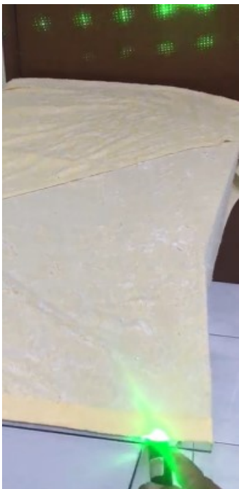
Fig. 3: Use blanket to cover the top surface of the glass and press the laser pen head with mounted spot pattern cap against glass width with partial head on top of glass surface
