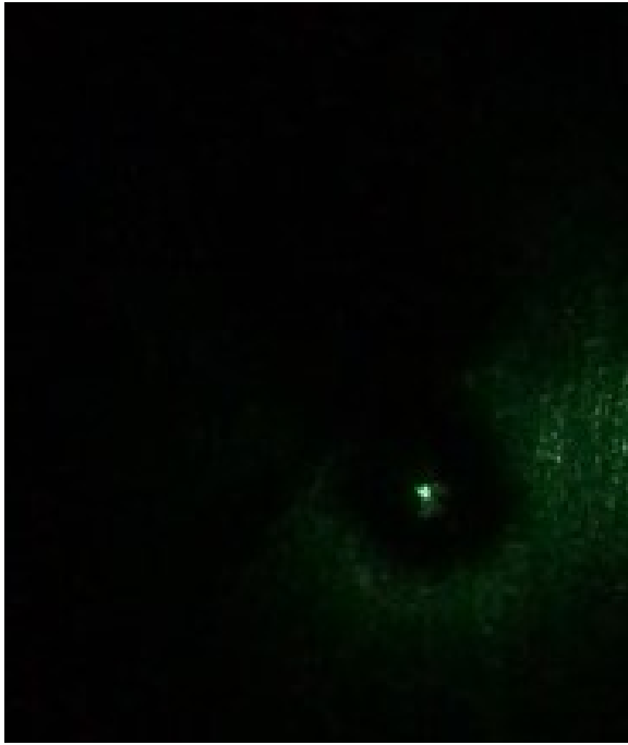
Fig. 9: A small light spot at the center of the small spherical seed's shadow
