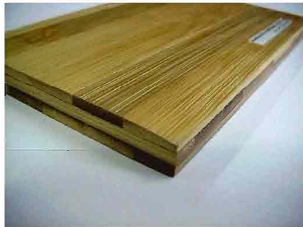
(A): Three-layers laminated bamboo
