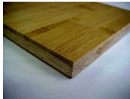
(B): Composite-ply consisting of a single layer Bamboo and two layers of wood veneers
