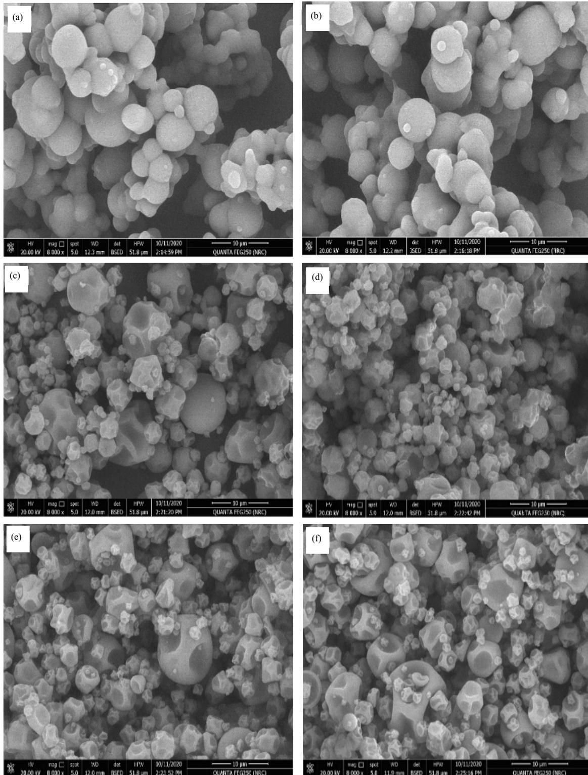
Fig. 1(a-f): Surface morphology of MPPE microcapsules
