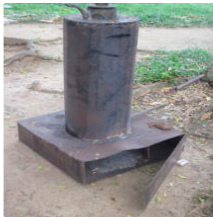
Fig. 3: The fabricated laboratory scale updraft gasifier
