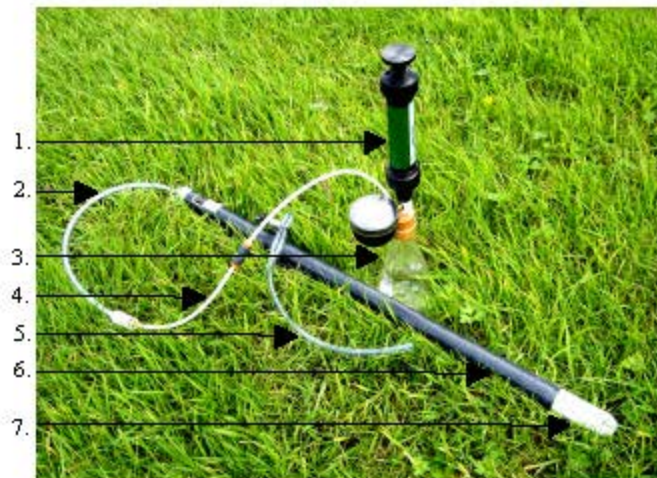
Fig 2: Ceramic cup assembly used at UCD, 2008. 1: Vacuum pump, 2: 10 mm Outer vacuum tube, 3: Sampling container, 4: 5 mm Sampling tube, 5: Vacuum tube extension, 6: PVC pipe and 7: Ceramic cup
