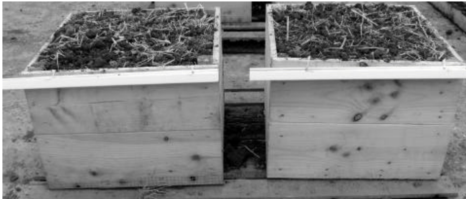
Fig. 1: Soil boxes used to determine the influence of measurement methodology on the recorded infiltration rate of a medium clay-loam soil
