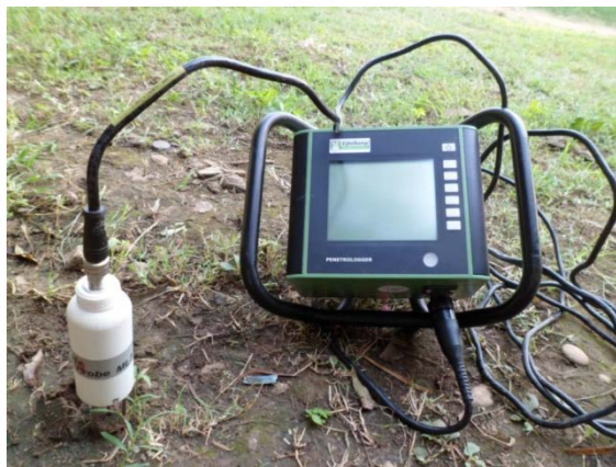
Fig. 3: Eijkelkamp Theta moisture sensor attached to the penetrometer display to read out real time soil moisture content
