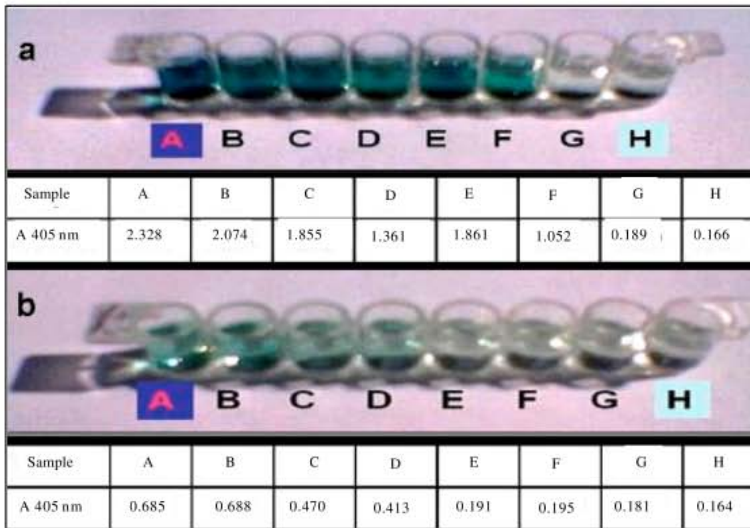
Fig. 5: Colorimetric detection of (a) DIG-labelled PLRV and (b) PVX-cDNA (b) products as shown by absorbance values of each assay. A: Positive control, B to G: Potato samples and H: Negative control
