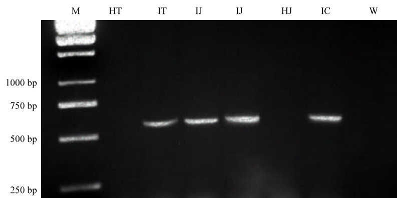
Fig. 2: A photograph of gel electrophoresis showing PCR products (~575 bp) amplified from the DNA-A of JMIV and other begomoviruses used as controls. Sizes of molecular weight markers (250 to 1000 bp) are shown on the left. M = 1 kb molecular weight marker (MBI Fermentas Life Sciences, Germany), HT = Healthy Tomato, IT = Tomato leaf curl virus-infected tomato, IJ = JMIV-infected Jatropha, HJ = Healthy Jatropha, IC = Cassava mosaic virus-infected cassava and W = Water control
