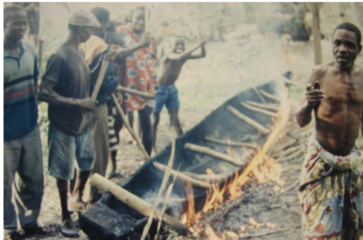
Fig. 1: Construction of a small canoe (dugout) from a tree using fire and water
