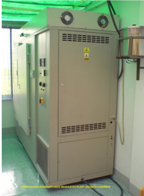
Fig. 1: Temperature-humidity-photoperiod controlled plant growth chamber (Source: Professor Dr. Mohammed Al-Amin)
