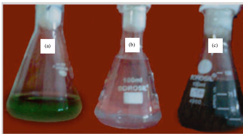
Fig. 1: Synthesis of nanoparticle using silver nitrate and leaf extract of Andrographis paniculata a: Leaf extract, b: 1 mM AgNO 3 without leaf extract and c: 1 mM AgNO 3 with 10% leaf extract after 5 h
