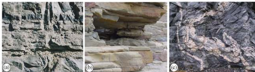
Fig. 1: Different types of stone or rock (a) limestone, (b) sandstone and (c) schist
