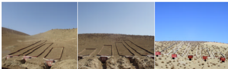
Fig. 2: Three kinds of experimental runoff measurement plots in different conditions
