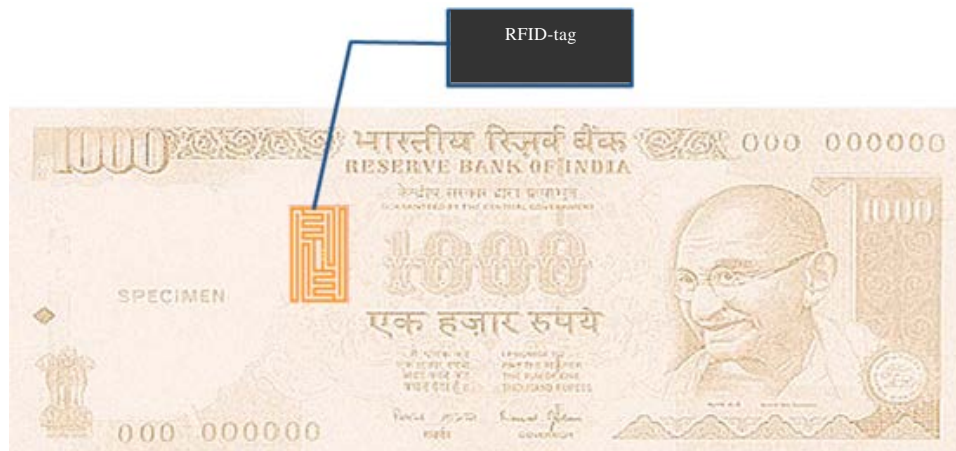
Fig. 3: Currency note equipped with RFID-Tag (currency note made of polymer)
