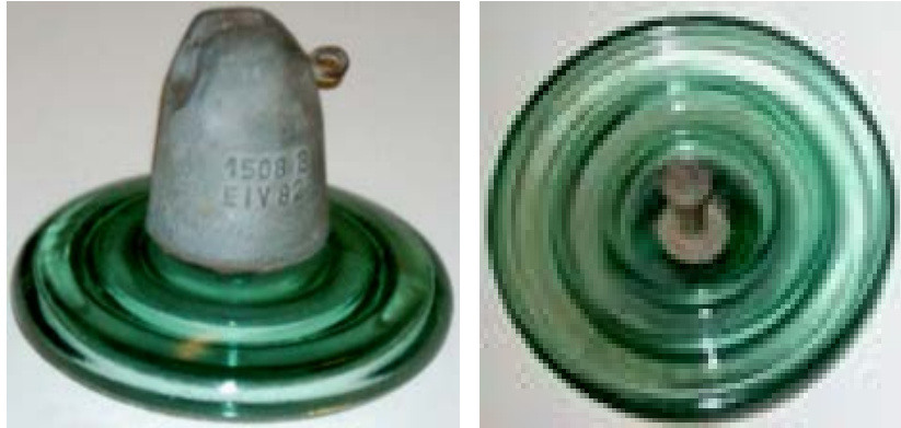
Fig. 7: A photographs showing a link of an insulator string
