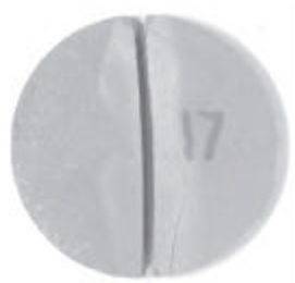
Fig. 4: Good failure in a Brazilian test that has subsequently generated a second crack Boukhalifa and James (2008)
