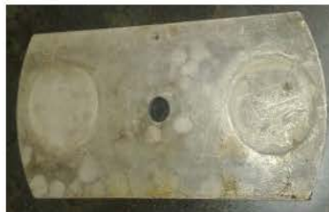
Fig. 10: A bonnet of the cell of a curing chamber
