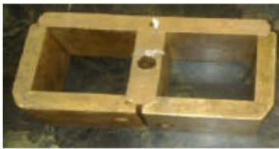
Fig. 8: Assembled sample cell of a curing chamber
