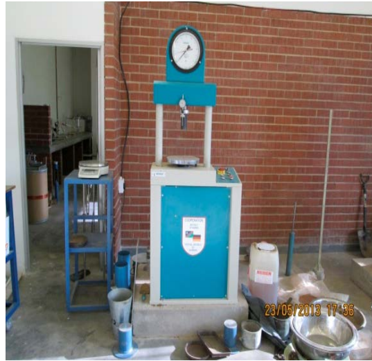
Fig. 6: California bearing ratio testing equipment
