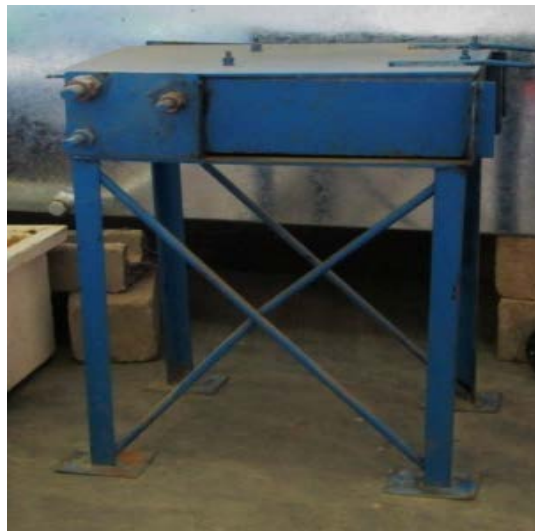
Fig. 7: Brick making mould used to produce the brick testing samples
