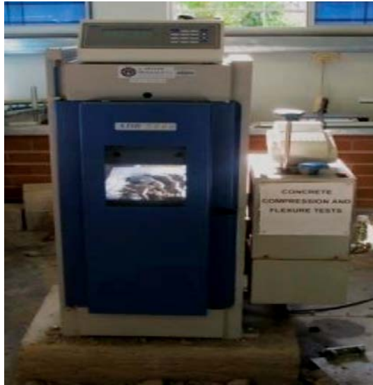
Fig. 8: Compression testing equipment used to measure the compressive strength of the test samples
