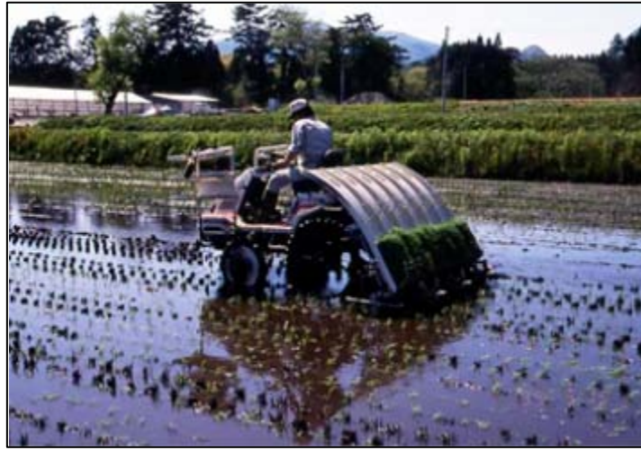
Fig. 2: Transplanting by a non-tillage transplanter
