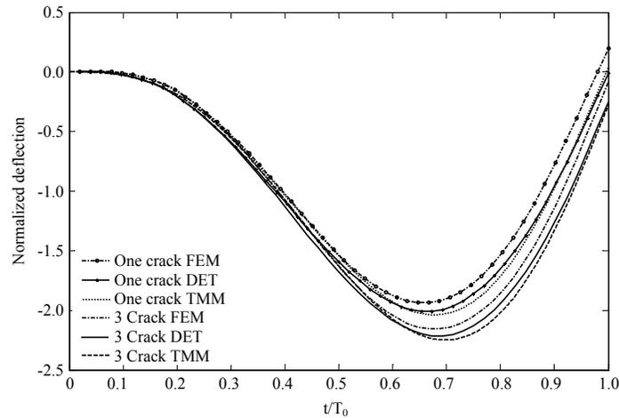
Fig. 5: Comparison of beam midpoint deflection for one and three cracks, TMM: Transfer matrix method, DET: Discrete element technique, FEM: Finite element method
