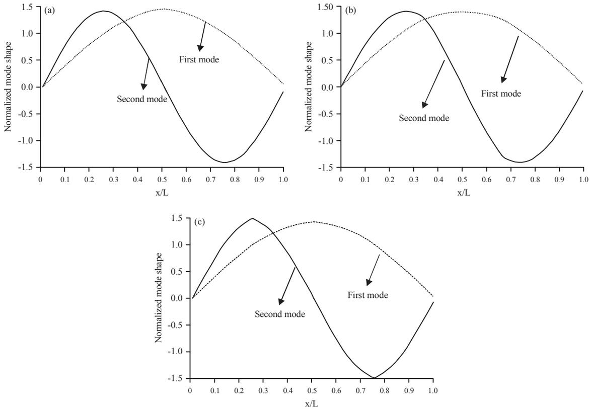
Fig. 9(a-c): First and second mode shapes of the beam with, (a) One crack in the middle, (b) Two cracks and (c) Three cracks
