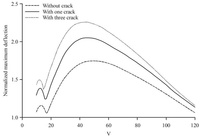
Fig. 11: Maximum normalized deflection versus mass speed for different numbers of cracks in the beam
