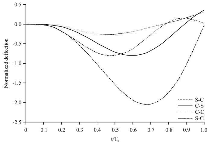
Fig. 6: Normalized deflection of mid-span for different boundary conditions in the beam with one crack in the middle
