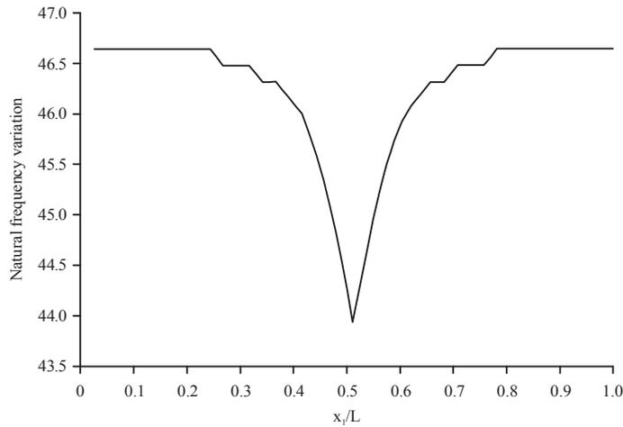
Fig. 8: Recording of first natural frequency for different crack locations
