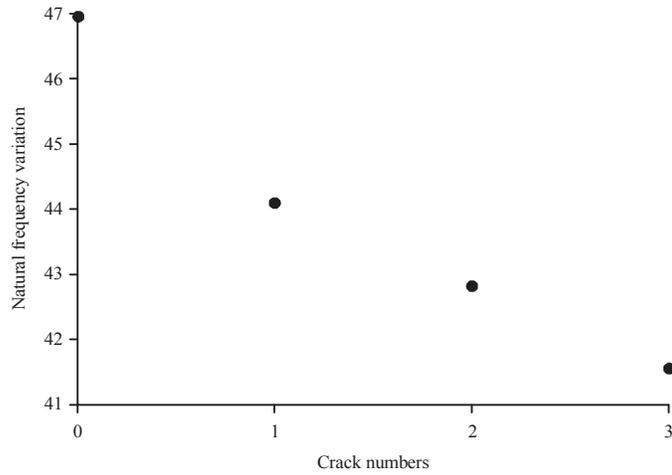
Fig. 7: Decrease of natural frequency with increasing numbers of crack
