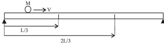
Fig. 3: Beam with two cracks
