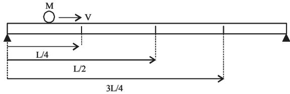
Fig. 4: Beam with three cracks
