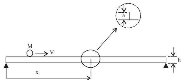
Fig. 1: Cracked beam under moving mass
