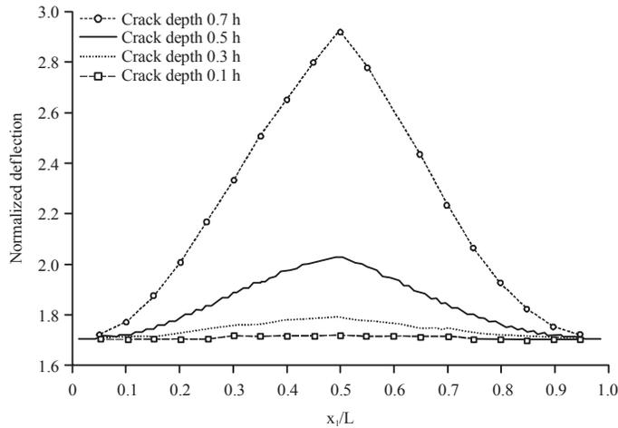
Fig. 10: Maximum normalized deflection versus crack locations for different crack depths
