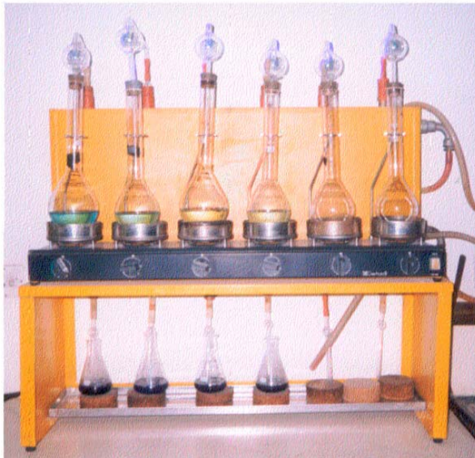
Fig. 1: Macro Kjeldhal distillation apparatus (for protein and NPN and TN analysis)
