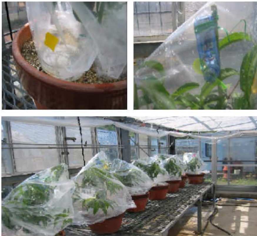
Fig. 12: Photo shows ^{13}\text{CO}_2 feeding in potted ( \phi 30 cm) one-year-old peach trees from 9-12 pm on July 31, 2003. A = Petri dish containing BaCO 3 with 50% lactic acid, B = Small fan to circulate air in the bag. C = Potted peach trees covered with transparent polyethylene bags
