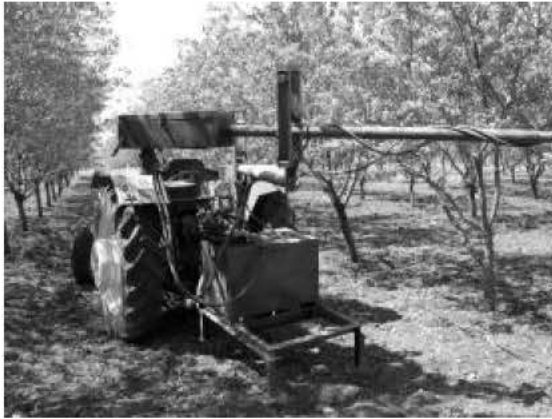
Fig. 2: The limb shaker used for almond harvesting
