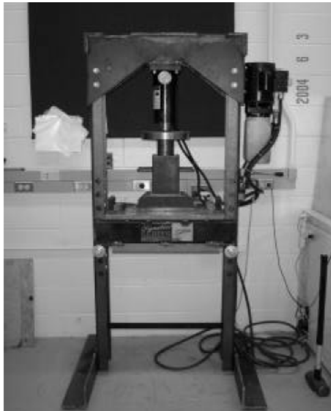
Fig. 1: The hydraulic press and the chamber used for the experiments
