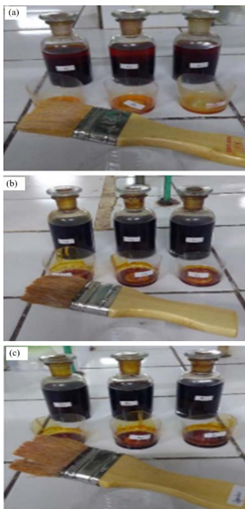
Fig. 1(a-c): Appearance of produced varnish from Ambalau resin extracted with (a) Methanol, (b) Ethanol and (c) Dan acetone
