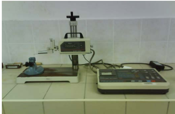
Fig. 2: Mitutoyo surfest SV-400 measuring instrument
