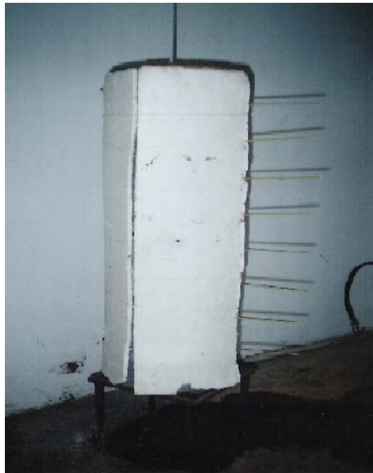
Fig. 1: Naturally aerated press mud bed
