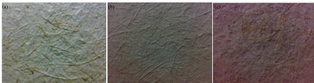
Fig. 1(a-c): Samples according to the mixtures, (a) 25% of coir fibers and 65% news, (b) 45% of coir fibers and 55% news and (c) 65% of coir fibers and 35% news
