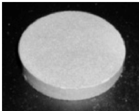
Fig. 3: Solid biomass fuel briquette of 10 g, 40 mm diameter
