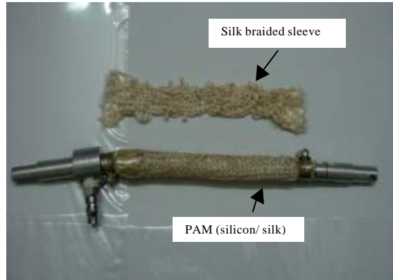
Fig. 4: Pneumatics muscle and silk braided sleeve (Krishna et al. , 2011)
