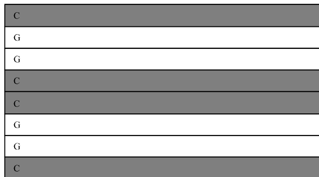
Fig. 1: Symmetrical design of HFRE composite
