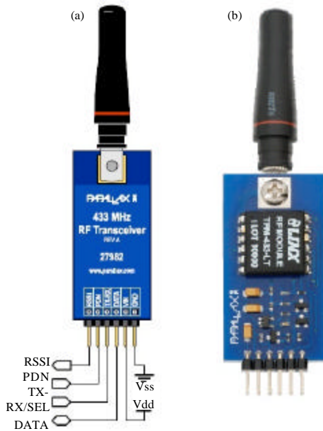
Fig. 5(a-b): Physical illustration of RF transceiver
