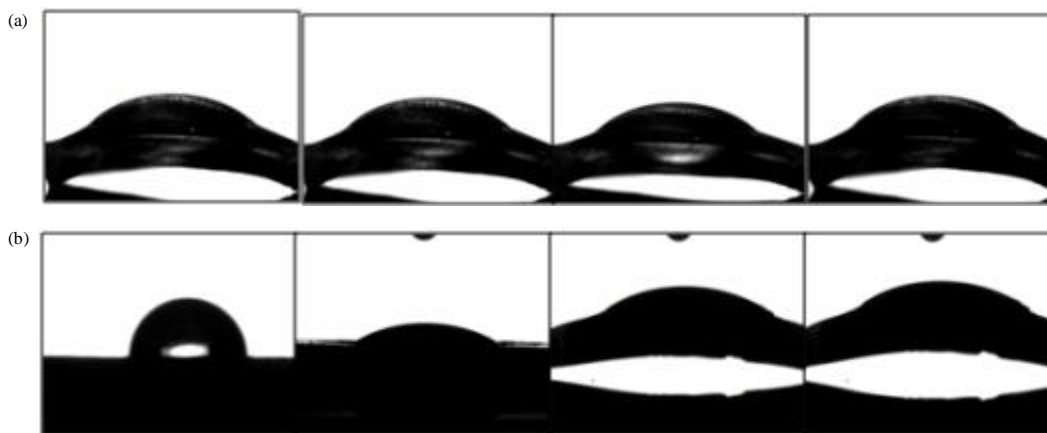
Fig. 4(a-b): Photographs showing the absorption of a water droplet with time (a) By a dry pristine PAM gel and (b) By a 0.01% MWNT/PAM composite gel
