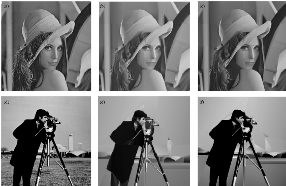
Fig. 10(a-f): (a) Original Lena. (512×512), (b) Reconstructed Lena using the GW algorithm (with tiling), 0.0625 bpp, PSNR = 28.72, (c) Reconstructed Lena using the proposed method (without tiling), 0.0625 bpp, PSNR = 29.78, (d) Original cameraman. (256×256). (e) Reconstructed cameraman using the GW algorithm (with tiling), 0.0625 bpp, PSNR = 22.93, (f) Reconstructed cameraman using the proposed method (without tiling), 0.0625 bpp, PSNR = 24.63
