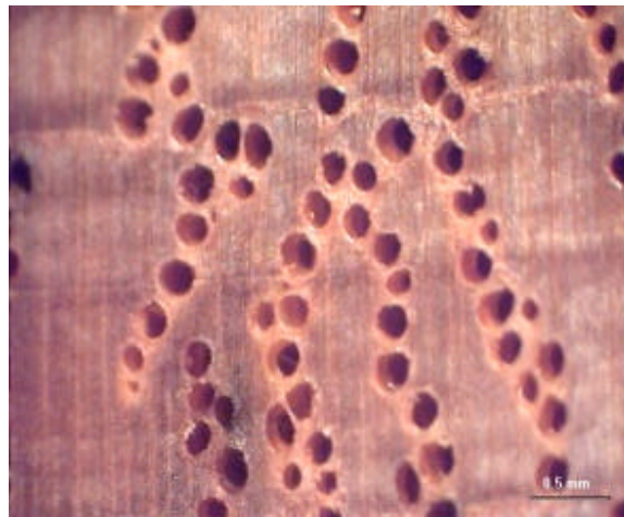
Fig. 3: Saninten ( Castanopsis sp.) Wood sample, identified from the anatomy of cross sectional area
